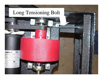
Use a ½" socket wrench to tighten the tensioning bolt just enough to remove the slipping. Check the tension on the belt that runs from the motor to the front roller by twisting or wiggling it. You should be able to twist the belt about 90 degrees.
